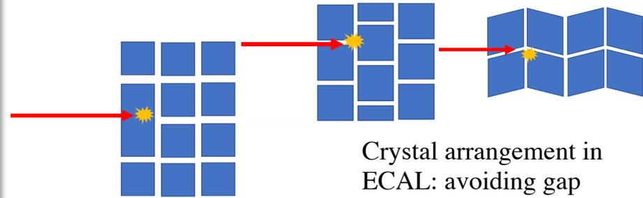
Crystal arrangement in ECAL: avoiding gap region; increased complexity in shower shape reconstruction.
