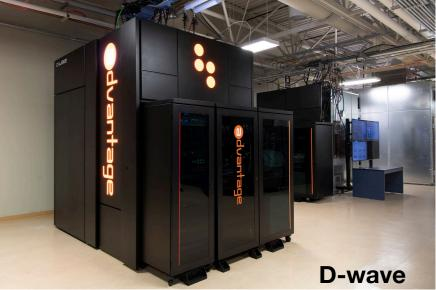
Temperature: below $1.5 \times 10^{-2}$ K dimension:  $3m \times 2.1m \times 3m$ Weight: 3800kg Power: (max) 25kW
