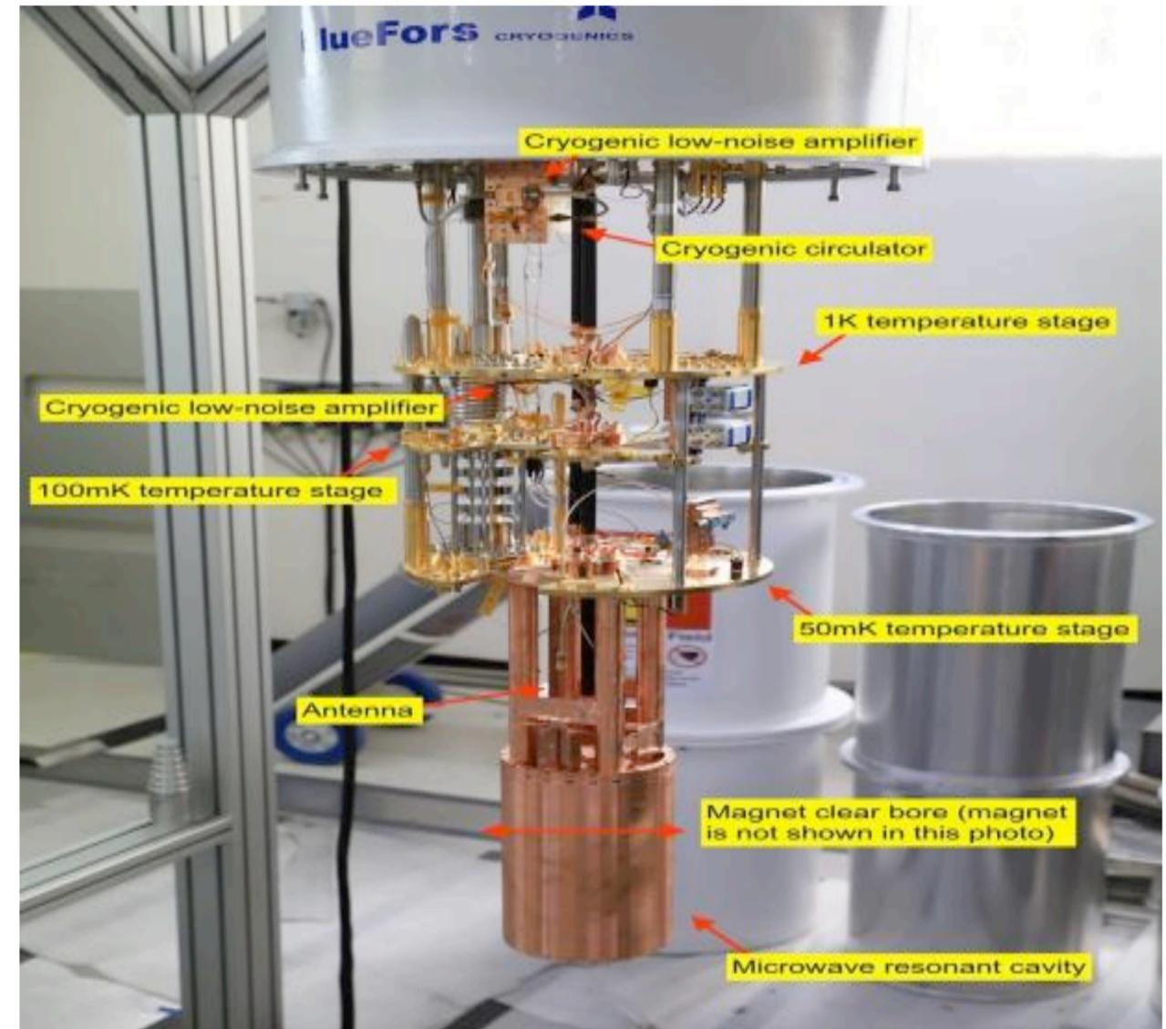
Electromagnetic Cavity in IBS-CAPP
