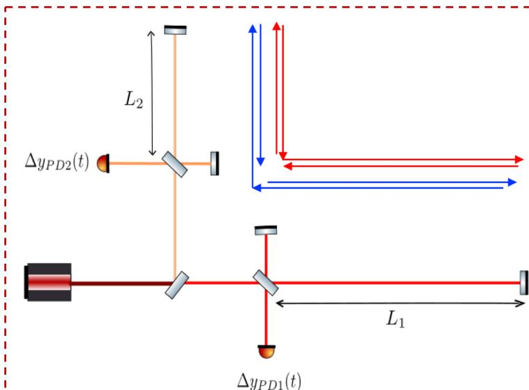
$$\begin{aligned}\Delta y_{PD1}(t) &= H_1(t) + p(t - T_1) - p(t), \\ \Delta y_{PD2}(t) &= H_2(t) + p(t - T_2) - p(t),\end{aligned}$$
